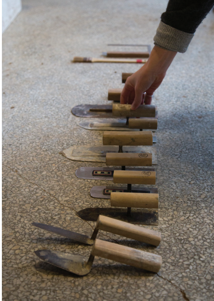
ABOVE: A COLLECTION OF TOOLS UTILIZED BY JAPANESE PLASTERERS IN EARTHEN WALL CONSTRUCTION
